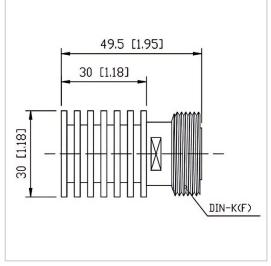
RF Solution offer a wide selection of Coaxial Fixed Termination (Dummy Load) for global customers. CT-10W-RA3030-DINK-4G is a Coaxial Fixed Termination (Dummy Load) in Frequency Range of DC~4.0 GHz. It is made of high quality materials under a high standard, the Connector Type of this product is DIN-F (K), VSWR Max is 1.25 and Impedance is 50  $\Omega$ . The component has a good working performance and stability, it is ideal for handling a Power of 10 W.
