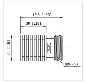
RF Solution offer a wide selection of Coaxial Fixed Termination (Dummy Load) for global customers. CT-10W-RA3030-DINK-3G is a Coaxial Fixed Termination (Dummy Load) in Frequency Range of DC~3.0 GHz. It is made of high quality materials under a high standard, the Connector Type of this product is DIN-F (K), VSWR Max is 1.20 and Impedance is 50  $\Omega$ . The component has a good working performance and stability, it is ideal for handling a Power of 10 W.
