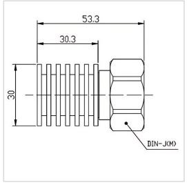
RF Solution offer a wide selection of Coaxial Fixed Termination (Dummy Load) for global customers. CT-10W-RA3030-DINJ-6G is a Coaxial Fixed Termination (Dummy Load) in Frequency Range of DC $\sim$ 6.0 GHz. It is made of high quality materials under a high standard, the Connector Type of this product is DIN-M (J), VSWR Max is 1.30 and Impedance is 50  $\Omega$ . The component has a good working performance and stability, it is ideal for handling a Power of 10 W.
