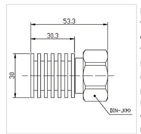
RF Solution offer a wide selection of Coaxial Fixed Termination (Dummy Load) for global customers. CT-10W-RA3030-DINJ-4G is a Coaxial Fixed Termination (Dummy Load) in Frequency Range of DC~4.0 GHz. It is made of high quality materials under a high standard, the Connector Type of this product is DIN-M (J), VSWR Max is 1.25 and Impedance is 50  $\Omega$ . The component has a good working performance and stability, it is ideal for handling a Power of 10 W.
