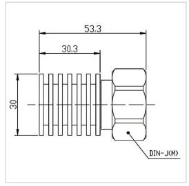
RF Solution offer a wide selection of Coaxial Fixed Termination (Dummy Load) for global customers. CT-10W-RA3030-DINJ-3G is а Coaxial Termination (Dummy Load) in Frequency Range of DC~3.0 GHz. It is made of high quality materials under a high standard, the Connector Type of this product is DIN-M (J), VSWR Max is 1.20 and Impedance is 50  $\Omega$ . The component has a good working performance and stability, it is ideal for handling a Power of 10 W.
