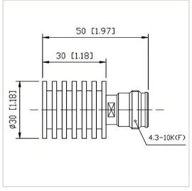
RF Solution offer a wide selection of Coaxial Fixed Termination (Dummy Load) for global customers. CT-10W-RA3030-4310K-6G is a Coaxial Termination (Dummy Load) in Frequency Range of DC~6.0 GHz. It is made of high quality materials under a high standard, the Connector Type of this product is 4.3-10-F (K), VSWR Max is 1.30 and Impedance is 50  $\Omega$ . The component has a good working performance and stability, it is ideal for handling a Power of 10 W.
