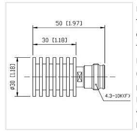
RF Solution offer a wide selection of Coaxial Fixed Termination (Dummy Load) for global customers. CT-10W-RA3030-4310K-4G is a Coaxial Fixed Termination (Dummy Load) in Frequency Range of DC~4.0 GHz. It is made of high quality materials under a high standard, the Connector Type of this product is 4.3-10-F (K), VSWR Max is 1.30 and Impedance is 50  $\Omega$ . The component has a good working performance and stability, it is ideal for handling a Power of 10 W.
