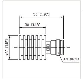
RF Solution offer a wide selection of Coaxial Fixed Termination (Dummy Load) for global customers. CT-10W-RA3030-4310K-3G is a Coaxial Fixed Termination (Dummy Load) in Frequency Range of DC~3.0 GHz. It is made of high quality materials under a high standard, the Connector Type of this product is 4.3-10-F (K), VSWR Max is 1.25 and Impedance is 50  $\Omega$ . The component has a good working performance and stability, it is ideal for handling a Power of 10 W.
