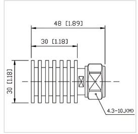
RF Solution offer a wide selection of Coaxial Fixed Termination (Dummy Load) for global customers. CT-10W-RA3030-4310J-6G is a Coaxial Fixed Termination (Dummy Load) in Frequency Range of DC~6.0 GHz. It is made of high quality materials under a high standard, the Connector Type of this product is 4.3-10-M (J), VSWR Max is 1.30 and Impedance is 50  $\Omega$ . The component has a good working performance and stability, it is ideal for handling a Power of 10 W.
