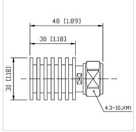
RF Solution offer a wide selection of Coaxial Fixed Termination (Dummy Load) for global customers. CT-10W-RA3030-4310J-4G is a Coaxial Fixed Termination (Dummy Load) in Frequency Range of DC~4.0 GHz. It is made of high quality materials under a high standard, the Connector Type of this product is 4.3-10-M (J), VSWR Max is 1.30 and Impedance is 50  $\Omega$ . The component has a good working performance and stability, it is ideal for handling a Power of 10 W.
