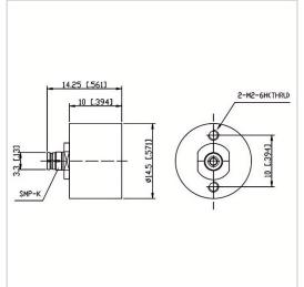
RF Solution offer a wide selection of Coaxial Fixed Termination (Dummy Load) for global customers. CT-10W-RA1015-SMPK-18G is a Coaxial Fixed Termination (Dummy Load) in Frequency Range of DC~18.0 GHz. It is made of high quality materials under a high standard, the Connector Type of this product is DIN-F (K), VSWR Max is 1.50 and Impedance is 50  $\Omega$ . The component has a good working performance and stability, it is ideal for handling a Power of 10 W.
