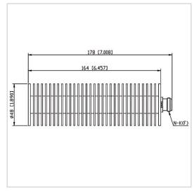
RF Solution offer a wide selection of Coaxial Fixed Termination (Dummy Load) for global customers. CT-100W-RA4816-NK-18G is a Coaxial Fixed Termination (Dummy Load) in Frequency Range of DC~18.0 GHz. It is made of high quality materials under a high standard, the Connector Type of this product is N-F (K), VSWR Max is 1.45 and Impedance is 50  $\Omega$ . The component has a good working performance and stability, it is ideal for handling a Power of 100 W.
