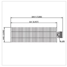
RF Solution offer a wide selection of Coaxial Fixed Termination (Dummy Load) for global customers. CT-100W-RA4816-NJ-18G is a Coaxial Fixed Termination (Dummy Load) in Frequency Range of DC~18.0 GHz. It is made of high quality materials under a high standard, the Connector Type of this product is N-M (J), VSWR Max is 1.45 and Impedance is 50  $\Omega$ . The component has a good working performance and stability, it is ideal for handling a Power of 100 W.
