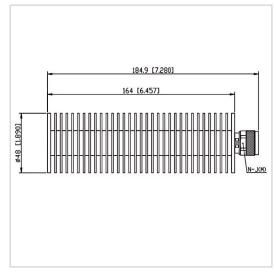
RF Solution offer a wide selection of Coaxial Fixed Termination (Dummy Load) for global customers. CT-100W-RA4816-NJ-12.4G is a Coaxial Fixed Termination (Dummy Load) in Frequency Range of DC~12.4 GHz. It is made of high quality materials under a high standard, the Connector Type of this product is N-M (J), VSWR Max is 1.35 and Impedance is 50  $\Omega$ . The component has a good working performance and stability, it is ideal for handling a Power of 100 W.
