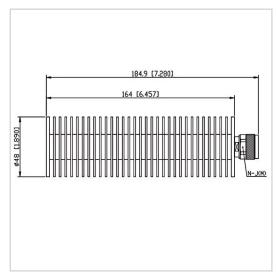
RF Solution offer a wide selection of Coaxial Fixed Termination (Dummy Load) for global customers. CT-100W-RA4816-NJ-10G is a Coaxial Fixed Termination (Dummy Load) in Frequency Range of DC~10.0 GHz. It is made of high quality materials under a high standard, the Connector Type of this product is N-M (J), VSWR Max is 1.30 and Impedance is 50  $\Omega$ . The component has a good working performance and stability, it is ideal for handling a Power of 100 W.
