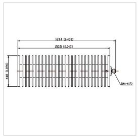
RF Solution offer a wide selection of Coaxial Fixed Termination (Dummy Load) for global customers. CT-100W-RA4815-SK-18G is a Coaxial Fixed Termination (Dummy Load) in Frequency Range of DC~18.0 GHz. It is made of high quality materials under a high standard, the Connector Type of this product is SMA-F (K), VSWR Max is 1.45 and Impedance is 50  $\Omega$ . The component has a good working performance and stability, it is ideal for handling a Power of 100 W.
