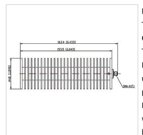
RF Solution offer a wide selection of Coaxial Fixed Termination (Dummy Load) for global customers. CT-100W-RA4815-SK-12.4G is a Coaxial Fixed Termination (Dummy Load) in Frequency Range of DC~12.4 GHz. It is made of high quality materials under a high standard, the Connector Type of this product is SMA-F (K), VSWR Max is 1.35 and Impedance is 50  $\Omega$ . The component has a good working performance and stability, it is ideal for handling a Power of 100 W.
