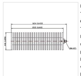
RF Solution offer a wide selection of Coaxial Fixed Termination (Dummy Load) for global customers. CT-100W-RA4815-SK-10G is a Coaxial Fixed Termination (Dummy Load) in Frequency Range of DC~8.0 GHz. It is made of high quality materials under a high standard, the Connector Type of this product is SMA-F (K), VSWR Max is 1.30 and Impedance is 50  $\Omega$ . The component has a good working performance and stability, it is ideal for handling a Power of 100 W.
