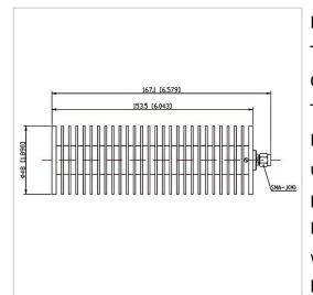
RF Solution offer a wide selection of Coaxial Fixed Termination (Dummy Load) for global customers. CT-100W-RA4815-SJ-18G is a Coaxial Fixed Termination (Dummy Load) in Frequency Range of DC~18.0 GHz. It is made of high quality materials under a high standard, the Connector Type of this product is SMA-M (J), VSWR Max is 1.45 and Impedance is 50  $\Omega$ . The component has a good working performance and stability, it is ideal for handling a Power of 100 W.
