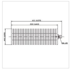
RF Solution offer a wide selection of Coaxial Fixed Termination (Dummy Load) for global customers. CT-100W-RA4815-SJ-12.4G is a Coaxial Fixed Termination (Dummy Load) in Frequency Range of DC~12.4 GHz. It is made of high quality materials under a high standard, the Connector Type of this product is SMA-M (J), VSWR Max is 1.35 and Impedance is 50  $\Omega$ . The component has a good working performance and stability, it is ideal for handling a Power of 100 W.
