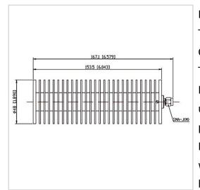
RF Solution offer a wide selection of Coaxial Fixed Termination (Dummy Load) for global customers. CT-100W-RA4815-SJ-10G is a Coaxial Fixed Termination (Dummy Load) in Frequency Range of DC~10.0 GHz. It is made of high quality materials under a high standard, the Connector Type of this product is SMA-M (J), VSWR Max is 1.30 and Impedance is 50  $\Omega$ . The component has a good working performance and stability, it is ideal for handling a Power of 100 W.
