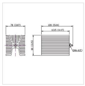
RF Solution offer a wide selection of Coaxial Fixed Termination (Dummy Load) for global customers. CT-100W-FA8011-SK-8G is a Coaxial Fixed Termination (Dummy Load) in Frequency Range of DC~8.0 GHz. It is made of high quality materials under a high standard, the Connector Type of this product is SMA-F (K), VSWR Max is 1.30 and Impedance is 50  $\Omega$ . The component has a good working performance and stability, it is ideal for handling a Power of 100 W.
