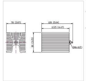
RF Solution offer a wide selection of Coaxial Fixed Termination (Dummy Load) for global customers. CT-100W-FA8011-SK-6G is a Coaxial Fixed Termination (Dummy Load) in Frequency Range of DC~6.0 GHz. It is made of high quality materials under a high standard, the Connector Type of this product is SMA-F (K), VSWR Max is 1.25 and Impedance is 50  $\Omega$ . The component has a good working performance and stability, it is ideal for handling a Power of 100 W.
