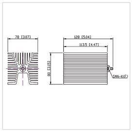
RF Solution offer a wide selection of Coaxial Fixed Termination (Dummy Load) for global customers. CT-100W-FA8011-SK-4G is Coaxial Termination (Dummy Load) in Frequency Range of DC~4.0 GHz. It is made of high quality materials under a high standard, the Connector Type of this product is SMA-F (K), VSWR Max is 1.25 and Impedance is 50  $\Omega$ . The component has a good working performance and stability, it is ideal for handling a Power of 100 W.
