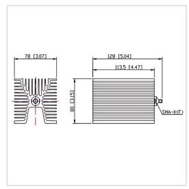
RF Solution offer a wide selection of Coaxial Fixed Termination (Dummy Load) for global customers. CT-100W-FA8011-SK-3G is Coaxial Termination (Dummy Load) in Frequency Range of DC~3.0 GHz. It is made of high quality materials under a high standard, the Connector Type of this product is SMA-F (K), VSWR Max is 1.20 and Impedance is 50  $\Omega$ . The component has a good working performance and stability, it is ideal for handling a Power of 100 W.
