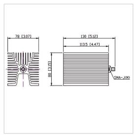
RF Solution offer a wide selection of Coaxial Fixed Termination (Dummy Load) for global customers. CT-100W-FA8011-SJ-8G is a Coaxial Fixed Termination (Dummy Load) in Frequency Range of DC~8.0 GHz. It is made of high quality materials under a high standard, the Connector Type of this product is SMA-M (J), VSWR Max is 1.30 and Impedance is 50  $\Omega$ . The component has a good working performance and stability, it is ideal for handling a Power of 100 W.
