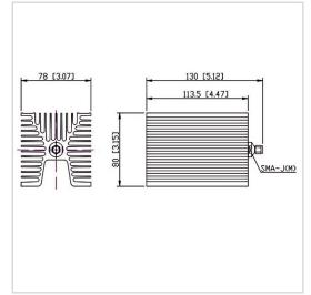
RF Solution offer a wide selection of Coaxial Fixed Termination (Dummy Load) for global customers. CT-100W-FA8011-SJ-6G is a Coaxial Fixed Termination (Dummy Load) in Frequency Range of DC~6.0 GHz. It is made of high quality materials under a high standard, the Connector Type of this product is SMA-M (J), VSWR Max is 1.25 and Impedance is 50  $\Omega$ . The component has a good working performance and stability, it is ideal for handling a Power of 100 W.
