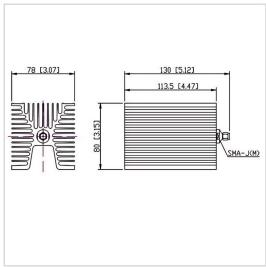
RF Solution offer a wide selection of Coaxial Fixed Termination (Dummy Load) for global customers. CT-100W-FA8011-SJ-4G is a Coaxial Fixed Termination (Dummy Load) in Frequency Range of DC~4.0 GHz. It is made of high quality materials under a high standard, the Connector Type of this product is SMA-M (J), VSWR Max is 1.25 and Impedance is 50  $\Omega$ . The component has a good working performance and stability, it is ideal for handling a Power of 100 W.
