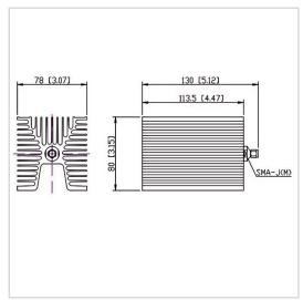
RF Solution offer a wide selection of Coaxial Fixed Termination (Dummy Load) for global customers. CT-100W-FA8011-SJ-3G is a Coaxial Fixed Termination (Dummy Load) in Frequency Range of DC $\sim$ 3.0 GHz. It is made of high quality materials under a high standard, the Connector Type of this product is SMA-M (J), VSWR Max is 1.20 and Impedance is 50  $\Omega$ . The component has a good working performance and stability, it is ideal for handling a Power of 100 W.
