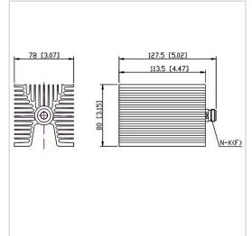
RF Solution offer a wide selection of Coaxial Fixed Termination (Dummy Load) for global customers. CT-100W-FA8011-NK-8G is a Coaxial Fixed Termination (Dummy Load) in Frequency Range of DC~8.0 GHz. It is made of high quality materials under a high standard, the Connector Type of this product is N-F (K), VSWR Max is 1.30 and Impedance is 50  $\Omega$ . The component has a good working performance and stability, it is ideal for handling a Power of 100 W.
