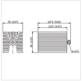
RF Solution offer a wide selection of Coaxial Fixed Termination (Dummy Load) for global customers. CT-100W-FA8011-NK-6G is a Coaxial Fixed Termination (Dummy Load) in Frequency Range of DC $\sim$ 6.0 GHz. It is made of high quality materials under a high standard, the Connector Type of this product is N-F (K), VSWR Max is 1.25 and Impedance is 50  $\Omega$ . The component has a good working performance and stability, it is ideal for handling a Power of 100 W.
