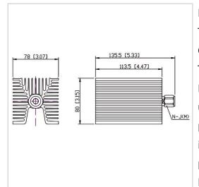
RF Solution offer a wide selection of Coaxial Fixed Termination (Dummy Load) for global customers. CT-100W-FA8011-NJ-8G is a Coaxial Fixed Termination (Dummy Load) in Frequency Range of DC~8.0 GHz. It is made of high quality materials under a high standard, the Connector Type of this product is N-M (J), VSWR Max is 1.30 and Impedance is 50  $\Omega$ . The component has a good working performance and stability, it is ideal for handling a Power of 100 W.
