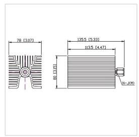
RF Solution offer a wide selection of Coaxial Fixed Termination (Dummy Load) for global customers. CT-100W-FA8011-NJ-6G is a Coaxial Fixed Termination (Dummy Load) in Frequency Range of DC $\sim$ 6.0 GHz. It is made of high quality materials under a high standard, the Connector Type of this product is N-M (J), VSWR Max is 1.25 and Impedance is 50  $\Omega$ . The component has a good working performance and stability, it is ideal for handling a Power of 100 W.
