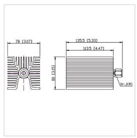
RF Solution offer a wide selection of Coaxial Fixed Termination (Dummy Load) for global customers. CT-100W-FA8011-NJ-4G is a Coaxial Fixed Termination (Dummy Load) in Frequency Range of DC~4.0 GHz. It is made of high quality materials under a high standard, the Connector Type of this product is N-M (J), VSWR Max is 1.25 and Impedance is 50  $\Omega$ . The component has a good working performance and stability, it is ideal for handling a Power of 100 W.
