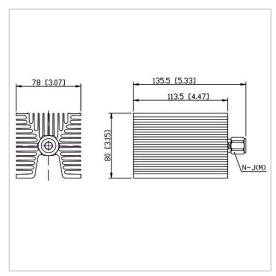
RF Solution offer a wide selection of Coaxial Fixed Termination (Dummy Load) for global customers. CT-100W-FA8011-NJ-3G is a Coaxial Fixed Termination (Dummy Load) in Frequency Range of DC $\sim$ 3.0 GHz. It is made of high quality materials under a high standard, the Connector Type of this product is N-M (J), VSWR Max is 1.20 and Impedance is 50  $\Omega$ . The component has a good working performance and stability, it is ideal for handling a Power of 100 W.
