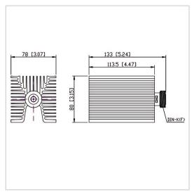
RF Solution offer a wide selection of Coaxial Fixed Termination (Dummy Load) for global customers. CT-100W-FA8011-DINK-6G is а Coaxial Termination (Dummy Load) in Frequency Range of DC~6.0 GHz. It is made of high quality materials under a high standard, the Connector Type of this product is DIN-F (K), VSWR Max is 1.30 and Impedance is 50  $\Omega$ . The component has a good working performance and stability, it is ideal for handling a Power of 100 W.
