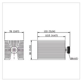
RF Solution offer a wide selection of Coaxial Fixed Termination (Dummy Load) for global customers. CT-100W-FA8011-DINK-3G is a Coaxial Fixed Termination (Dummy Load) in Frequency Range of DC $\sim$ 3.0 GHz. It is made of high quality materials under a high standard, the Connector Type of this product is DIN-F (K), VSWR Max is 1.20 and Impedance is 50  $\Omega$ . The component has a good working performance and stability, it is ideal for handling a Power of 100 W.
