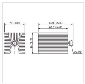
RF Solution offer a wide selection of Coaxial Fixed Termination (Dummy Load) for global customers. CT-100W-FA8011-4310K-4G is a Coaxial Fixed Termination (Dummy Load) in Frequency Range of DC~4.0 GHz. It is made of high quality materials under a high standard, the Connector Type of this product is 4.3-10-F (K), VSWR Max is 1.30 and Impedance is 50  $\Omega$ . The component has a good working performance and stability, it is ideal for handling a Power of 100 W.
