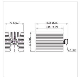
RF Solution offer a wide selection of Coaxial Fixed Termination (Dummy Load) for global customers. CT-100W-FA8011-4310K-3G is a Coaxial Fixed Termination (Dummy Load) in Frequency Range of DC~3.0 GHz. It is made of high quality materials under a high standard, the Connector Type of this product is 4.3-10-F (K), VSWR Max is 1.20 and Impedance is 50  $\Omega$ . The component has a good working performance and stability, it is ideal for handling a Power of 100 W.
