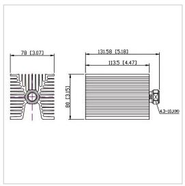
RF Solution offer a wide selection of Coaxial Fixed Termination (Dummy Load) for global customers. CT-100W-FA8011-4310J-6G is a Coaxial Fixed Termination (Dummy Load) in Frequency Range of DC~6.0 GHz. It is made of high quality materials under a high standard, the Connector Type of this product is 4.3-10-M (J), VSWR Max is 1.20 and Impedance is 50  $\Omega$ . The component has a good working performance and stability, it is ideal for handling a Power of 100 W.
