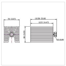
RF Solution offer a wide selection of Coaxial Fixed Termination (Dummy Load) for global customers. CT-100W-FA8011-4310J-4G is a Coaxial Fixed Termination (Dummy Load) in Frequency Range of DC~4.0 GHz. It is made of high quality materials under a high standard, the Connector Type of this product is 4.3-10-M (J), VSWR Max is 1.20 and Impedance is 50  $\Omega$ . The component has a good working performance and stability, it is ideal for handling a Power of 100 W.
