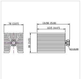
RF Solution offer a wide selection of Coaxial Fixed Termination (Dummy Load) for global customers. CT-100W-FA8011-4310J-3G is a Coaxial Fixed Termination (Dummy Load) in Frequency Range of DC $\sim$ 3.0 GHz. It is made of high quality materials under a high standard, the Connector Type of this product is 4.3-10-M (J), VSWR Max is 1.20 and Impedance is 50  $\Omega$ . The component has a good working performance and stability, it is ideal for handling a Power of 100 W.
