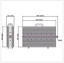
RF Solution offer a wide selection of Coaxial Fixed Termination (Dummy Load) for global customers. CT-1000W-FF3049-NK-1G is a Coaxial Fixed Termination (Dummy Load) in Frequency Range of DC~1.0 GHz. It is made of high quality materials under a high standard, the Connector Type of this product is N-F (K), VSWR Max is 1.35 and Impedance is 50  $\Omega$ . The component has a good working performance and stability, it is ideal for handling a Power of 1000 W.
