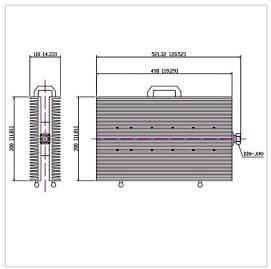
RF Solution offer a wide selection of Coaxial Fixed Termination (Dummy Load) for global customers. CT-1000W-FF3049-DINJ-3G is a Coaxial Fixed Termination (Dummy Load) in Frequency Range of DC $\sim$ 3.0 GHz. It is made of high quality materials under a high standard, the Connector Type of this product is DIN-M (J), VSWR Max is 1.35 and Impedance is 50  $\Omega$ . The component has a good working performance and stability, it is ideal for handling a Power of 1000 W.
