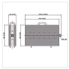
RF Solution offer a wide selection of Coaxial Fixed Termination (Dummy Load) for global customers. CT-1000W-FF3049-DINJ-2G is a Coaxial Fixed Termination (Dummy Load) in Frequency Range of DC~2.0 GHz. It is made of high quality materials under a high standard, the Connector Type of this product is DIN-M (J), VSWR Max is 1.35 and Impedance is 50  $\Omega$ . The component has a good working performance and stability, it is ideal for handling a Power of 1000 W.
