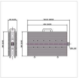
RF Solution offer a wide selection of Coaxial Fixed Termination (Dummy Load) for global customers. CT-1000W-FF3049-DINJ-1G is a Coaxial Fixed Termination (Dummy Load) in Frequency Range of DC~1.0 GHz. It is made of high quality materials under a high standard, the Connector Type of this product is DIN-M (J), VSWR Max is 1.35 and Impedance is 50  $\Omega$ . The component has a good working performance and stability, it is ideal for handling a Power of 1000 W.
