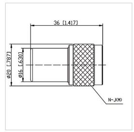
RF Solution offer a wide selection of Coaxial Fixed Termination (Dummy Load) for global customers. CT-05W-RF2036-NJ-4G is a Coaxial Fixed Termination (Dummy Load) in Frequency Range of DC~4.0 GHz. It is made of high quality materials under a high standard, the Connector Type of this product is N-M (J), VSWR Max is 1.25 and Impedance is 50  $\Omega$ . The component has a good working performance and stability, it is ideal for handling a Power of 5 W.
