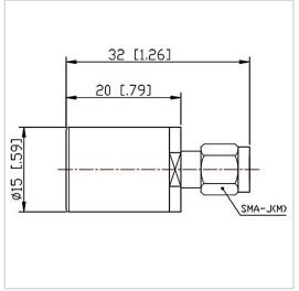
RF Solution offer a wide selection of Coaxial Fixed Termination (Dummy Load) for global customers. CT-05W-RF1520-SJ-4G is a Coaxial Fixed Termination (Dummy Load) in Frequency Range of DC~4.0 GHz. It is made of high quality materials under a high standard, the Connector Type of this product is SMA-M (J), VSWR Max is 1.25 and Impedance is 50  $\Omega$ . The component has a good working performance and stability, it is ideal for handling a Power of 5 W.
