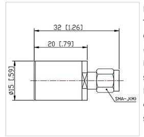
RF Solution offer a wide selection of Coaxial Fixed Termination (Dummy Load) for global customers. CT-05W-RF1520-SJ-3G is a Coaxial Fixed Termination (Dummy Load) in Frequency Range of DC $\sim$ 3.0 GHz. It is made of high quality materials under a high standard, the Connector Type of this product is SMA-M (J), VSWR Max is 1.20 and Impedance is 50  $\Omega$ . The component has a good working performance and stability, it is ideal for handling a Power of 5 W.
