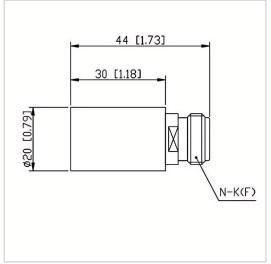
RF Solution offer a wide selection of Coaxial Fixed Termination (Dummy Load) for global customers. CT-05W-RA2030-NK-6G is a Coaxial Fixed Termination (Dummy Load) in Frequency Range of DC $\sim$ 6.0 GHz. It is made of high quality materials under a high standard, the Connector Type of this product is N-F (K), VSWR Max is 1.25 and Impedance is 50  $\Omega$ . The component has a good working performance and stability, it is ideal for handling a Power of 5 W.
